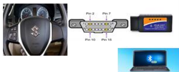
Fig. 1 Laptop is interfaced with Vehicle through ELM327
