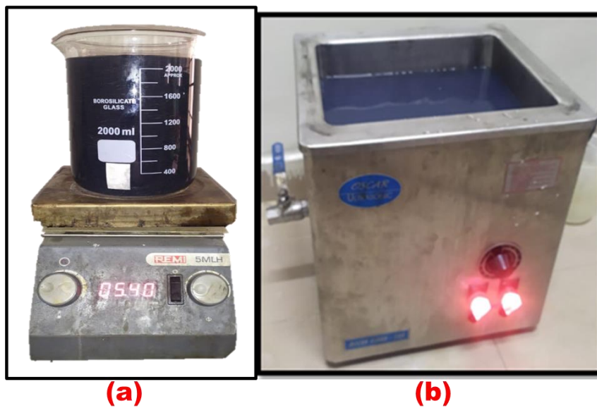
Fig. 2. (a) Magnetic stirrer, (b) Ultrasonic processor.
