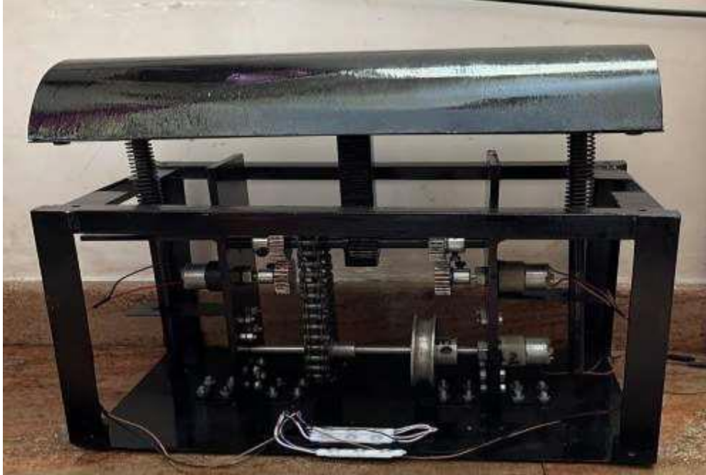
Figure: Developed model of Power Generation Model using Power Humps
